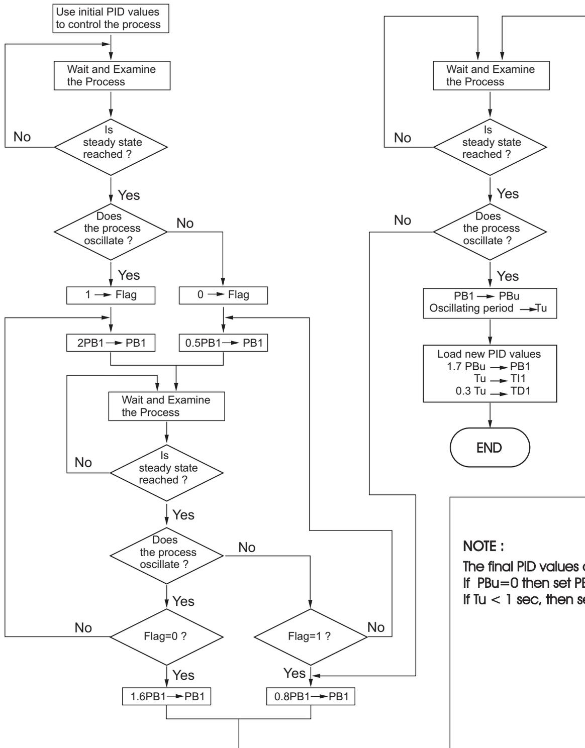
The above procedure may take a long time before reaching a new steady state since the P band was changed. This is particularly true for a slow process. So the above manual tuning procedures will take from minutes to hours to obtain optimal PID values.
