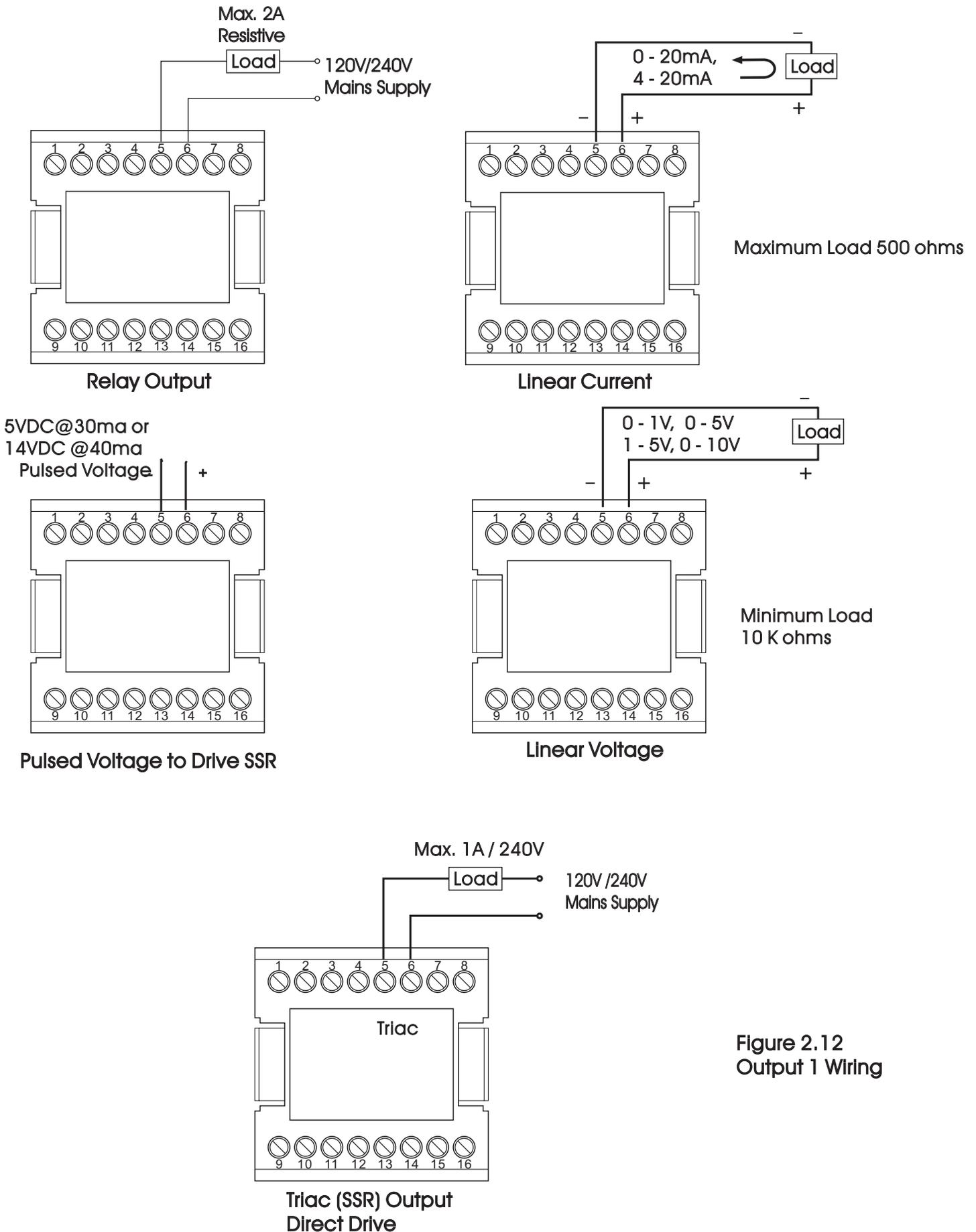
Figure 2.12 Output 1 Wiring
